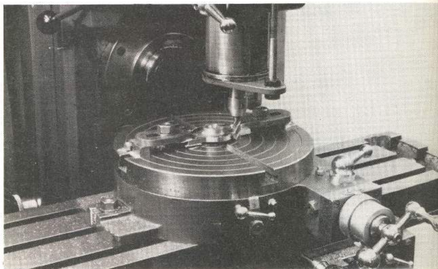
Fig. 15: Using the rotary table to profile the bottom cylinder cover.
